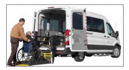
Body on Chassis Vehicle with lift (14- to 191-passenger; can be customized to include more wheelchair tie downs and reduce overall passenger count)
